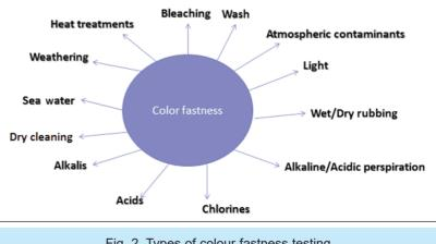
Fig. 2. Types of colour fastness testing
